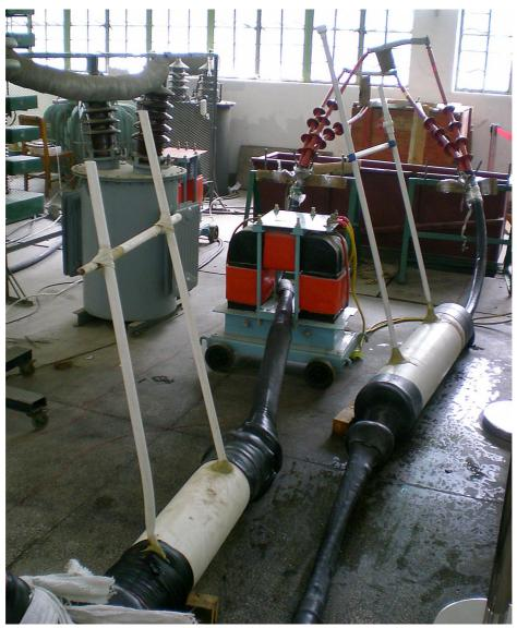
Complete set-up during heating cycle voltage test under water
