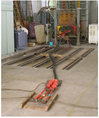
Complete set-up during thermal and dynamic short-circuit test
