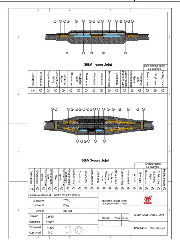
Note: Above drawing is for reference only, the final product is determined by negotiation based on cable construction and electrical requirements.
